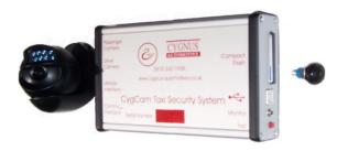
To turn the CygCam on, open the door of your vehicle or turn the ignition on. After a short (about 15 seconds) startup sequence, CygCam will record pictures and audio to memory. To signal that this has started, the indicator will flash red / green about once every second. Each flash shows that one photo has been taken.
