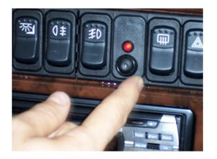
Your dealer will show you where the record button has been positioned. This allows you to make longer recordings should you feel it necessary. Three minutes before this button is pressed and up to five minutes afterwards will be saved. Normally two of these sequences can be held on the memory card. The indicator will go red during one of these recordings.
